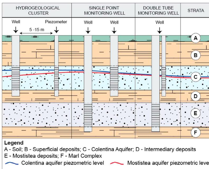
Figure 1 – Types of the groundwater monitoring stations
